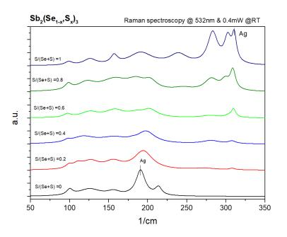
polycrystals were free from secondary phases. As expected for the same crystal structure of  $Sb_2Se_3$  and  $Sb_2S_3$ , the bimodal behavior of the main  $A_g$  Raman mode is detected.
